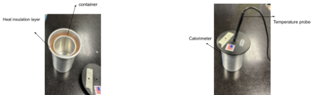
Figure 1: The calorimeter used in the experiment and its crucial parts.
